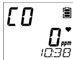
CO (carbon monoxide) gas concentration display
